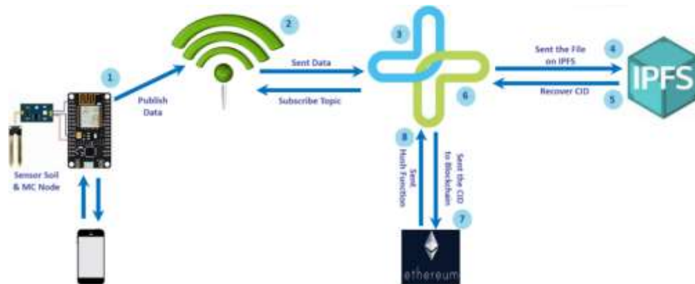
Figure 2. General structure of our proposed approach: It involves setting up an IoT system (irrigation system). This system sends data via the MQTT protocol. We integrated this system with a blockchain network and IPFS to secure the captured data against IoT attacks.
